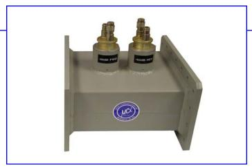
MCI's Directional Loop Couplers are designed to couple signals from a high power transmission line. The High Power Loop Coupler has an external load and can measure either forward or reverse power without rotation by manually repositioning the load. Directional couplers can be installed in all waveguide components (e.g. Bends, switches, ect.) in any combination of setting.
