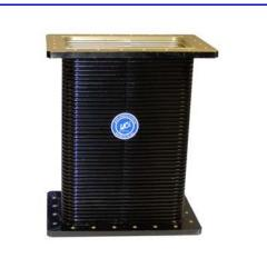
The MCI Flex Waveguide section allows for flexible movement in both the "E" and "H" planes. Flex sections are constructed of corrugated material and all seams are braze welded. Flat or gasket EIA flanges are then welded to both ends. All materials and surfaces are designed for long life under heavy loads. Various flex section lengths are available to custom fit the desired configuration.
