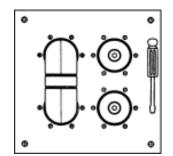
Manual transfer 5 pole patch panel assembly with (2) 180° elbows, includes 5 anchor connectors and 5 line clamps. Screwdriver mounted on panel. Not pressurized.
