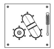
Manual transfer 4 pole patch panel assembly with (2) 180° elbows, includes 4 anchor connectors and 4 line clamps. Screwdriver mounted on panel. Not pressurized.
