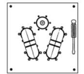
Manual transfer patch panel assembly 7 pole, three (3) 180° connectors, includes 7 anchor connectors and 7 line clamps. Screwdriver mounted on panel. Not pressurized.
