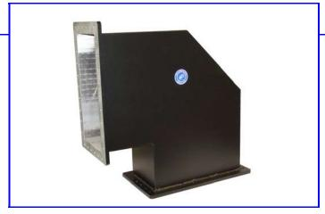
MCI designs and manufactures standard and custom miter bends in angles from 20 to 90 degrees. For angles less then 20, "Jogs" or "Flex waveguide can be utilized. Contact us regarding your application and we'll find the best solution. All bends are electrical optimized for superior electrical performance over a restricted bandwidth (typically VSWR 1.02:1 over a 10% bandwidth).
