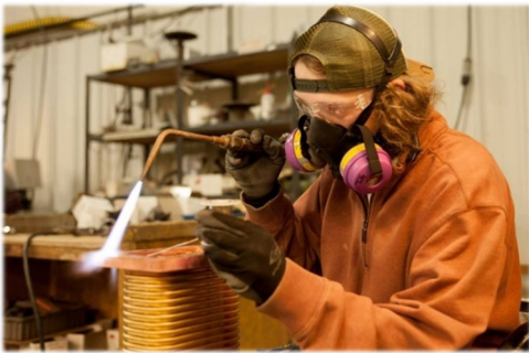
Brazing Flexible Waveguide
